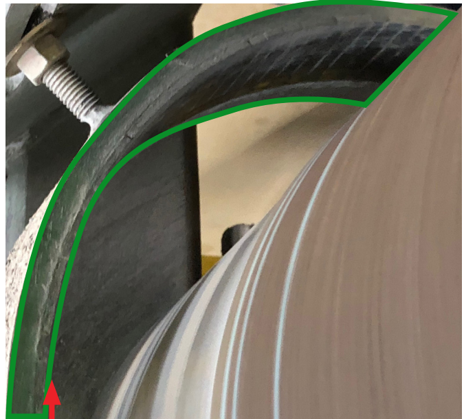
Above: GET 1/8" Tungsten Carbide lining the underside, still fully functioning after 31+ months
