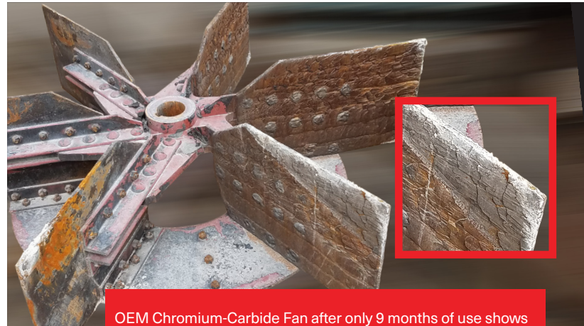
OEM Chromium-Carbide Fan after only 9 months of use shows severe wear and loss of operational and structural integrity.
