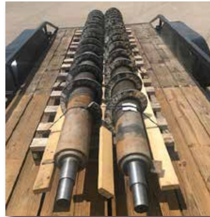
The GET Z-Screws each had more than 8,000 pieces of Carbide applied, and lasted more than 14 months!
