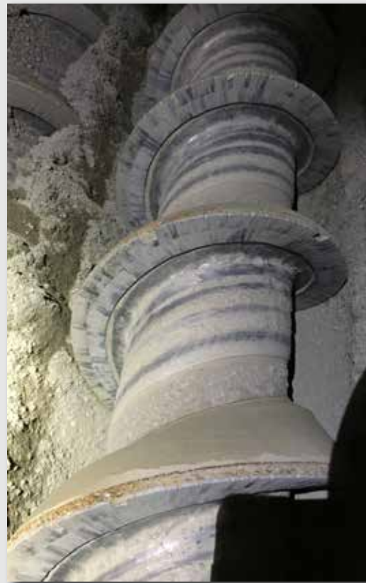
GET Carbide-protected Z-Screws are able to withstand the harsh environment of material handling.
