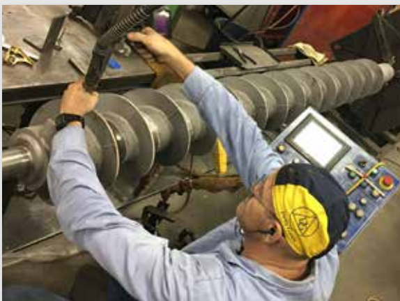
A skilled GET engineer quality checking a Tungsten Carbide protected Z-Screw in production.
