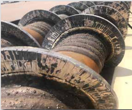
The combination of solid Tungsten Carbide and hardfacing has more than tripled the life of these feed screws.
