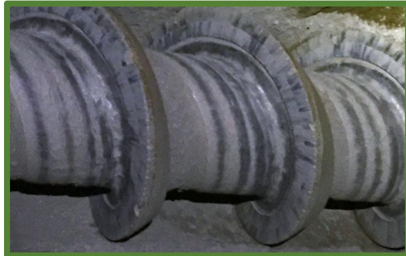
The 10 foot long 10-inch diameter Tungsten Carbide GET Z-Screw after 2 years of moving the same granulated mineral slag has maintained both push-face integrity and overall flight diameter.
