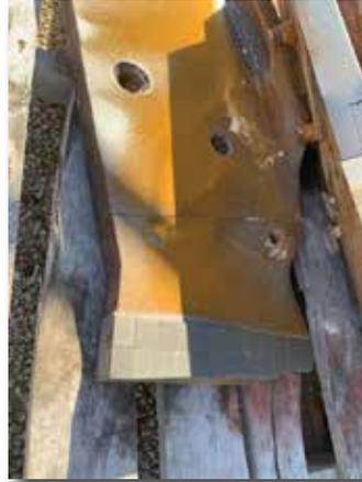
After almost a year, the GET Carbide-protected plow tip shows minimal wear.
