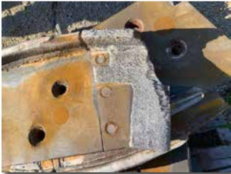
The hard-facing protection on the plow tips would wear off after just a few months.
