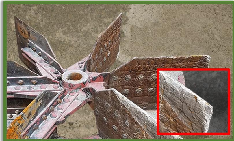
OEM Chromium-Carbide Fan after only 12 months of use shows severe wear and loss of operational and structural integrity.
