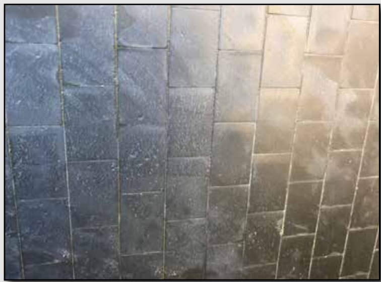
The GET Solid Tungsten Carbide-protected Transfer Hopper wear plate was able to withstand the harsh environment of material handling.
